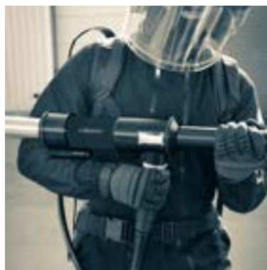
VT380.10/5 : small telescopic hydraulic jack
