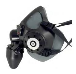
Automatic Ambient Air Valve enables unrestricted ambient air breathing. Automatically closes upon roll-over or water submersion. Automatically reopens upon up-righting or surfacing. Also includes manual override feature for operational testing.
